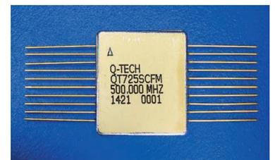
The QT725S VCSCO is a Class 2 hybrid per MILPRF-55310, hermetically sealed, and operated from  $-40^{\circ}\text{C}$  to  $+85^{\circ}\text{C}$ . Absolute Pull range (APR) is  $\pm 20\text{ppm}$  min.
